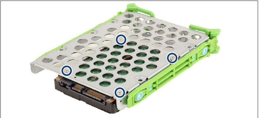
Figure 41: Attaching the 2.5-inch HDD to the 3.5-inch HDD carrier
