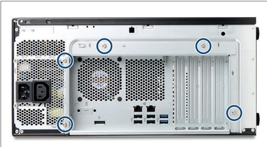
Figure 144: System board tray - Location of screws
