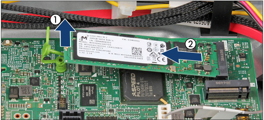
Figure 137: Removing the M.2 SSD (B)
