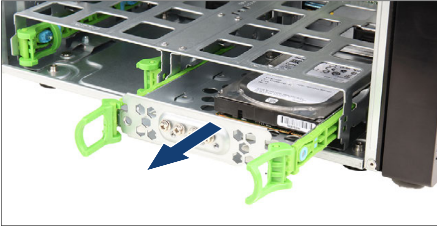
Figure 43: Removing a 2.5-inch HDD
