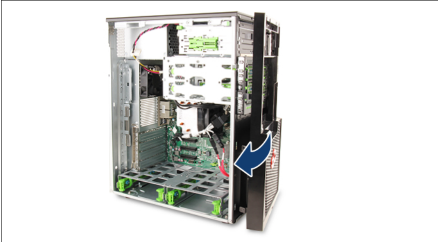
Figure 23: Installing the front cover (B)
