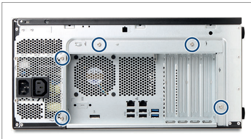
Figure 139: System board tray - Location of screws
