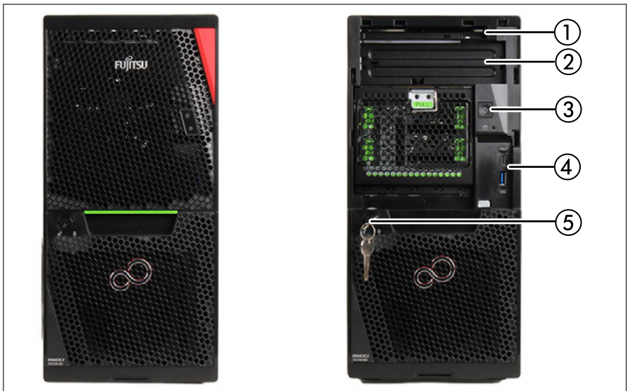
Figure 152: Server front with bay cover (left) and without bay cover (right)
