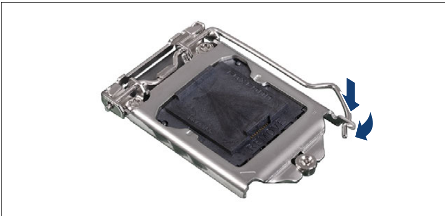
Figure 97: Latching the socket lever
