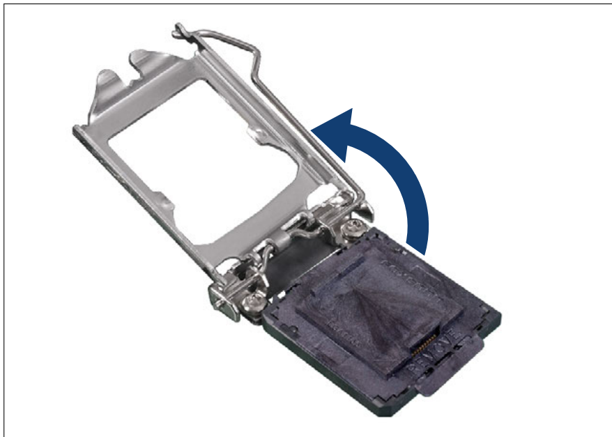
Figure 99: Opening the load plate
