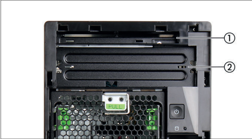
Figure 101: Accessible drive bays
