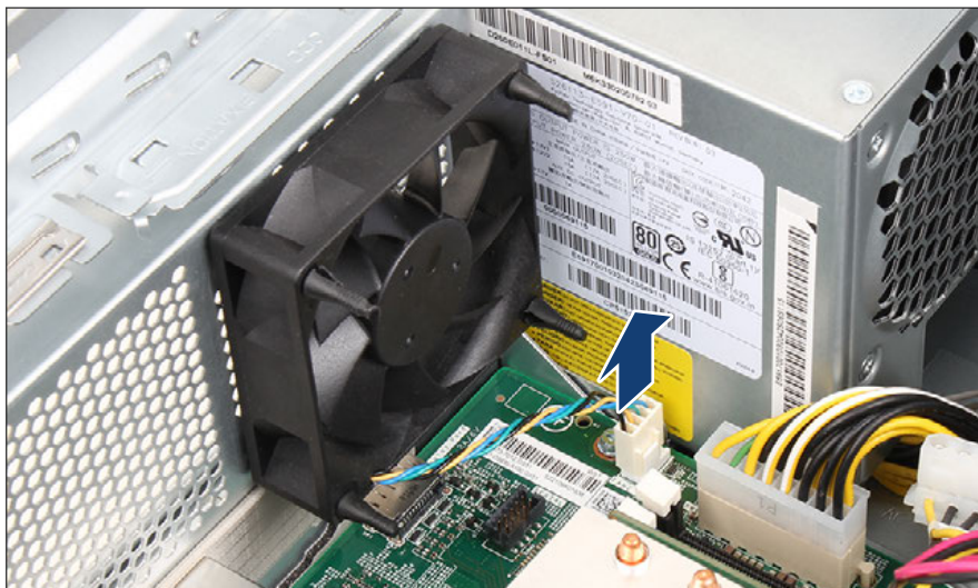
Figure 53: Disconnecting the rear fan cable
