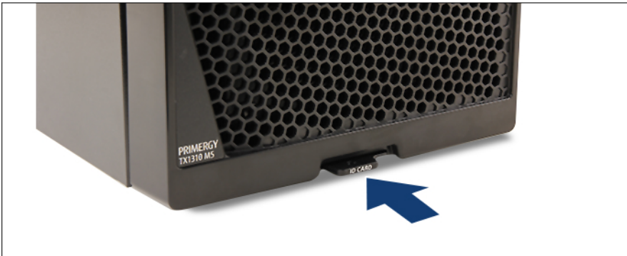
Figure 24: Installing the ID card
