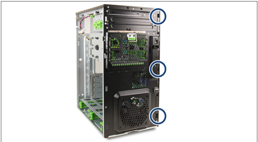
Figure 22: Installing the front cover (A)
