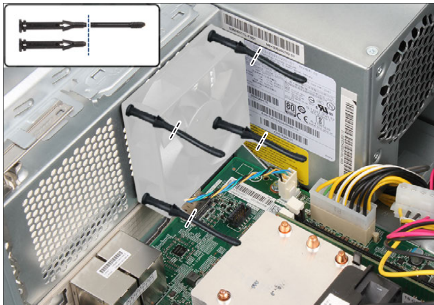
Figure 57: Cutting off the rubber rivets
