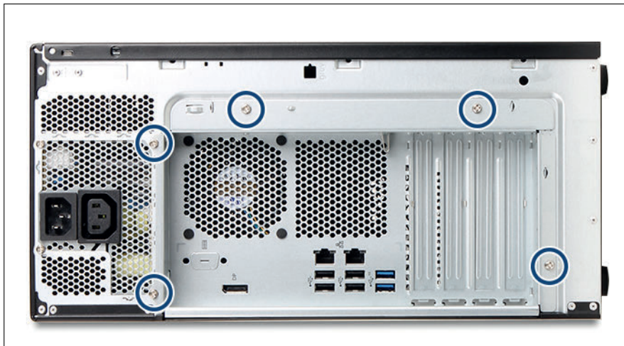
Figure 15: System board tray - Location of screws
