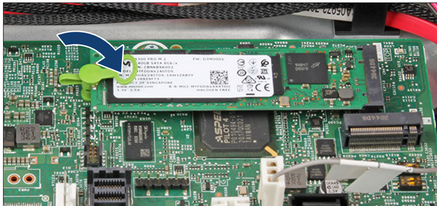
Figure 135: Installing the M.2 SSD (B)
