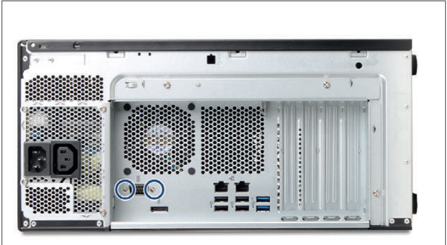
Figure 117: Installing the serial interface (B)
