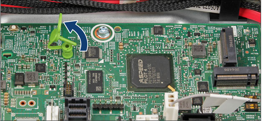
Figure 133: Opening the M.2 lock
