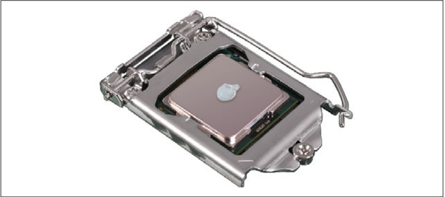
Figure 90: Applying the thermal paste
