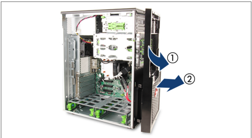
Figure 11: Removing the front cover (B)
