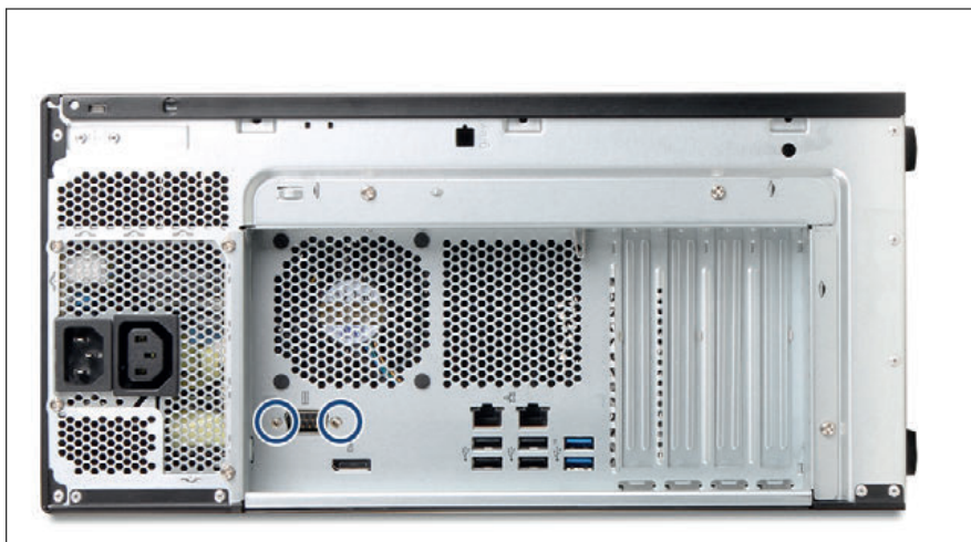
Figure 118: Removing the serial interface (A)
