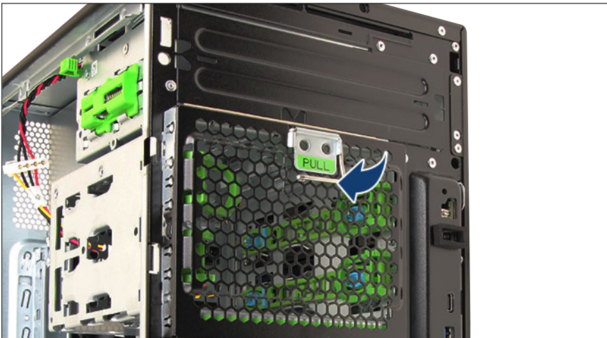
Figure 21: Folding down the lever
