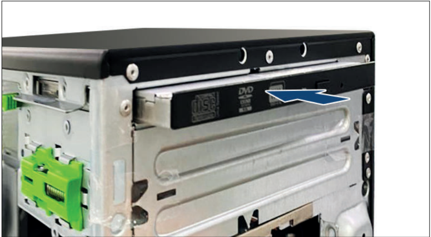
Figure 105: Installing the ODD
