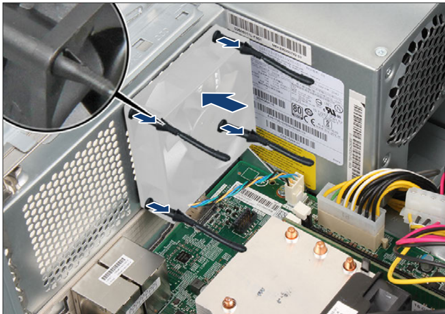
Figure 56: Installing the rear fan
