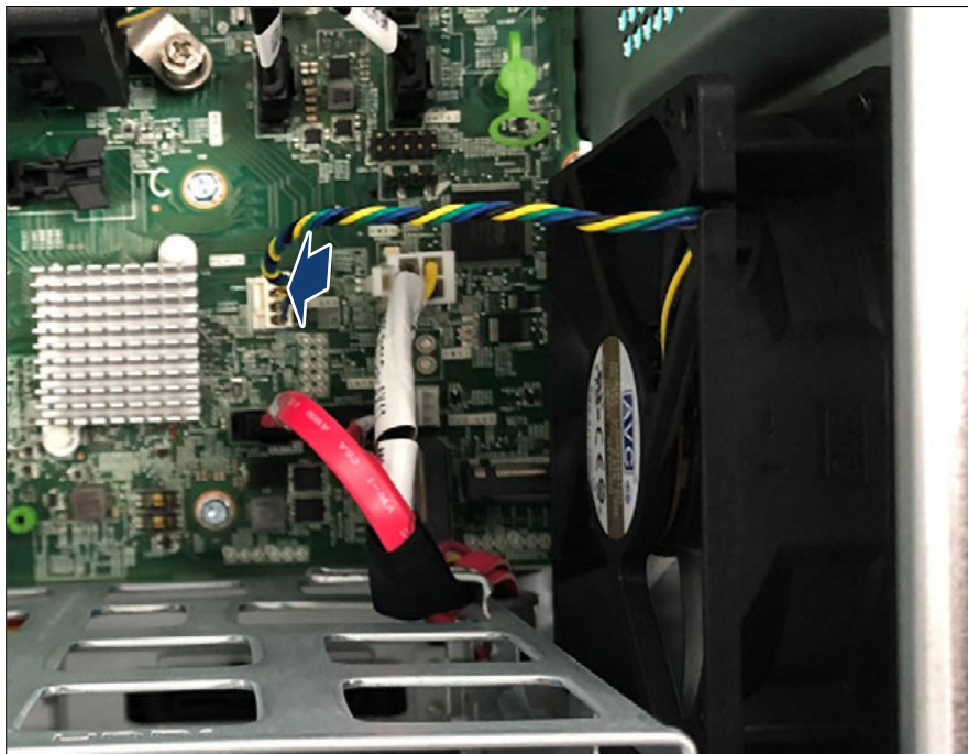
Figure 64: Connecting the front fan cable
