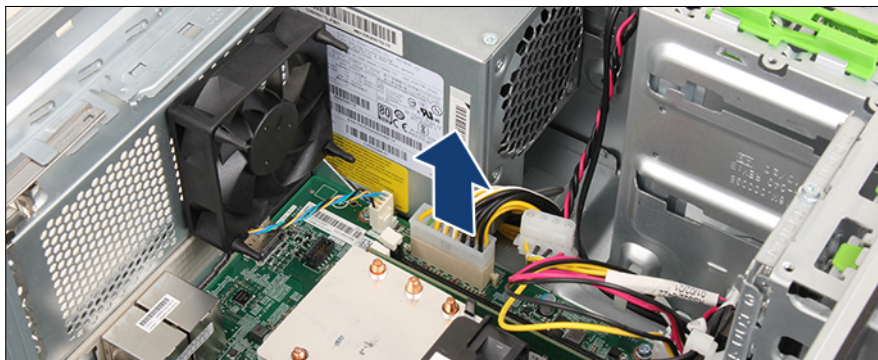
Figure 31: Disconnecting the power cable
