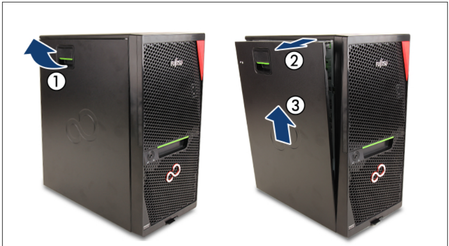
Figure 8: Removing the side cover
