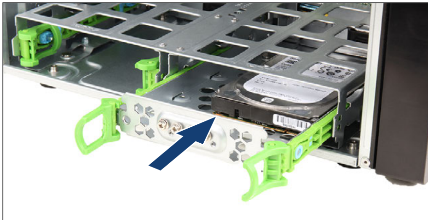
Figure 42: Installing a 2.5-inch HDD
