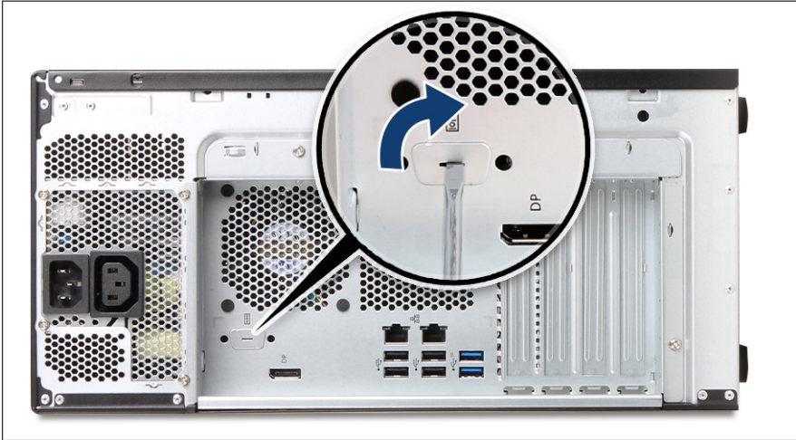
Figure 115: Removing the metal cover
