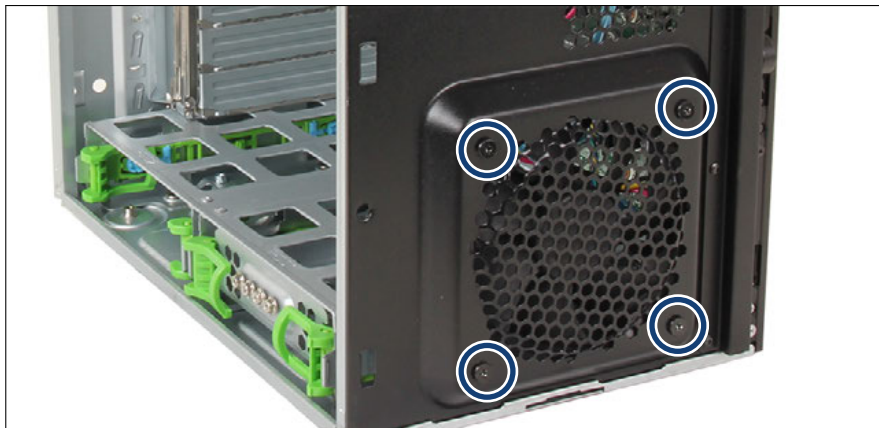
Figure 63: Fastening the screws
