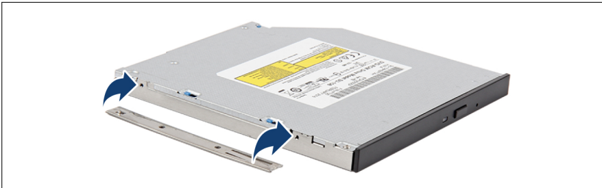
Figure 104: Attaching the fixation plate to the ODD
