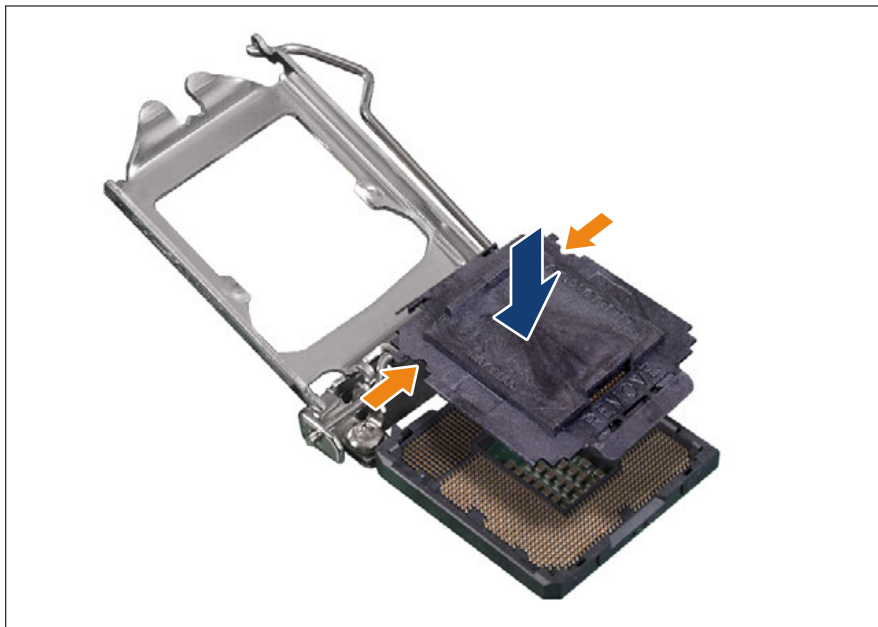
Figure 94: Attaching the protective socket cover
