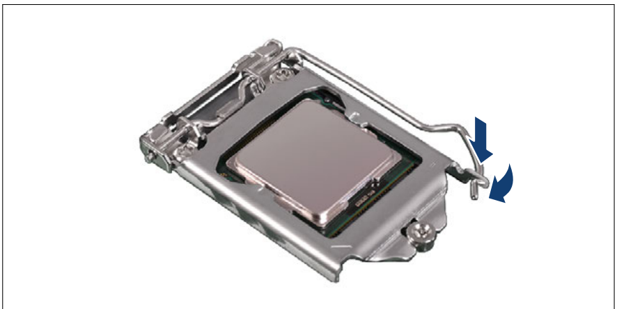
Figure 88: Closing the socket release lever
