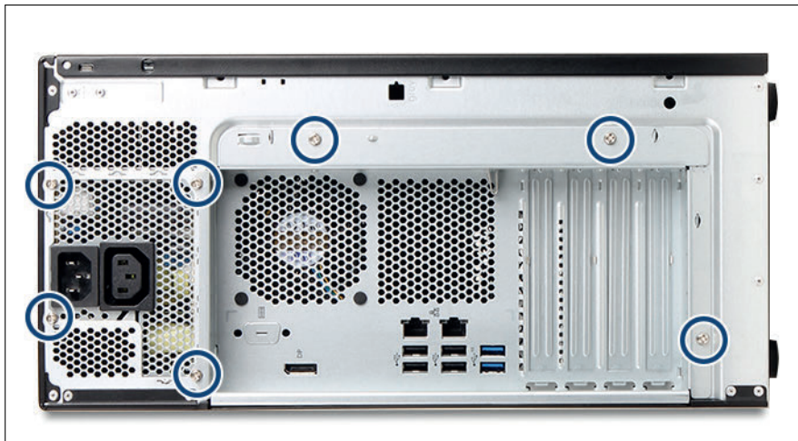
Figure 37: Fastening the screws
