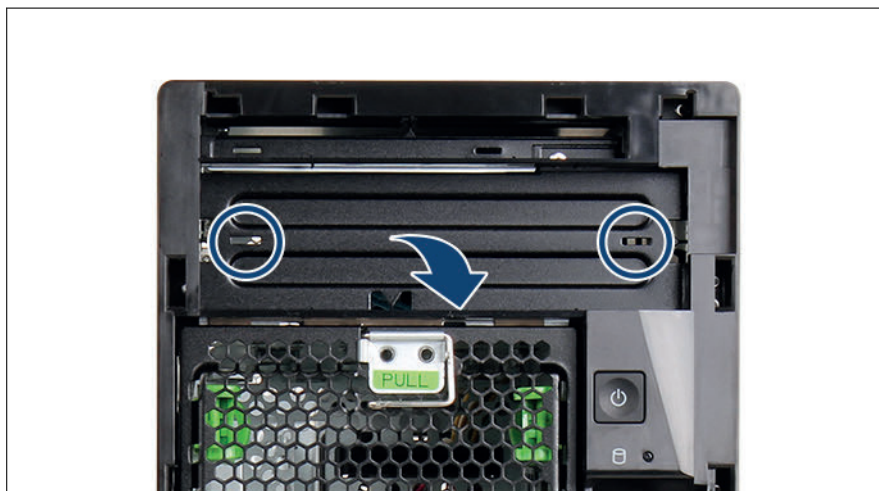
Figure 108: Removing the dummy cover bay 2
