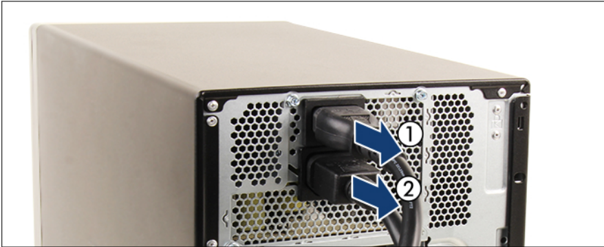
Figure 7: Disconnecting the power cords
