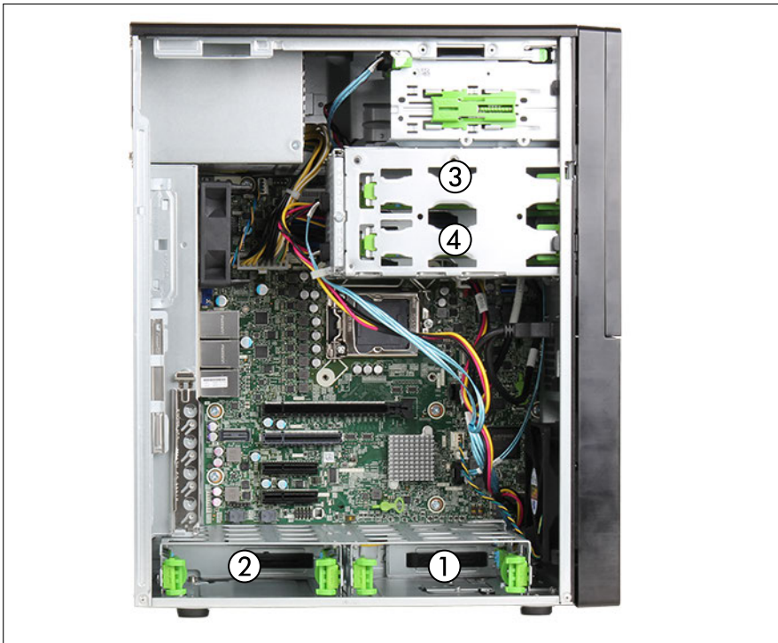
Figure 39: 3.5-inch HDD location
