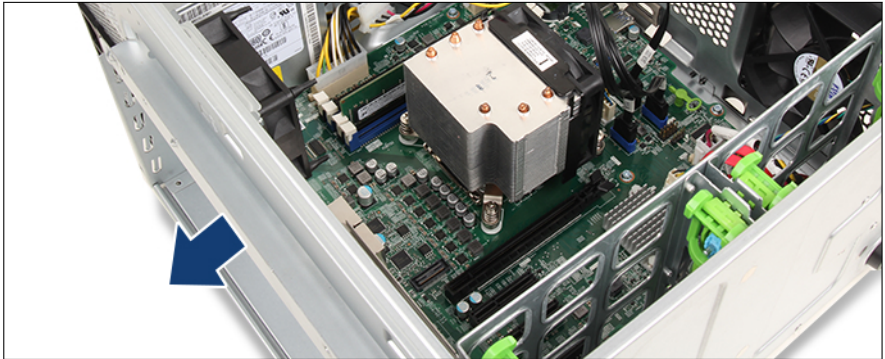
Figure 33: Pulling out the system board tray by 1-2 cm
