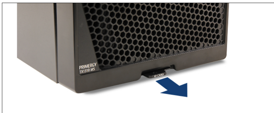
Figure 9: Removing the ID card
