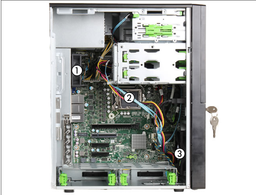
Figure 52: Positions of the system fans
