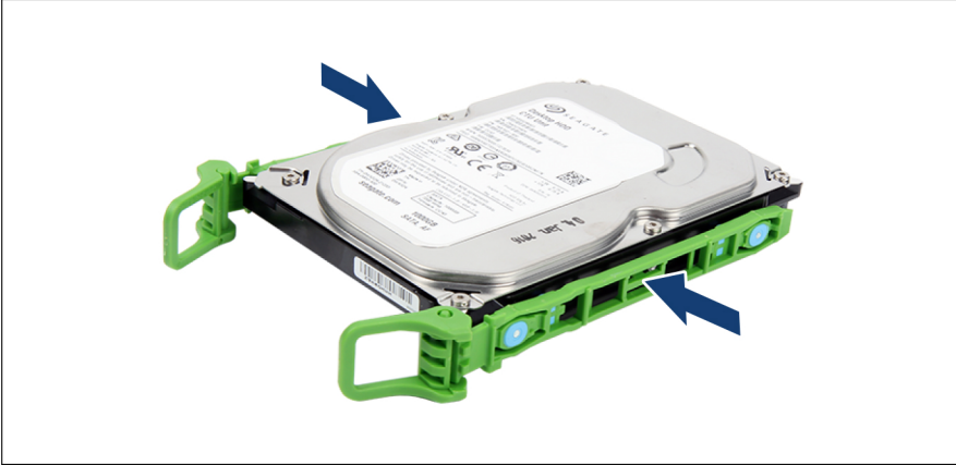
Figure 47: Attaching the Easyrails
