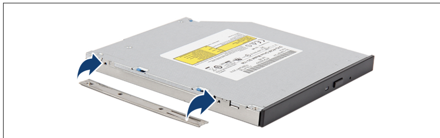
Figure 107: Attaching the fixation plate to the ODD
