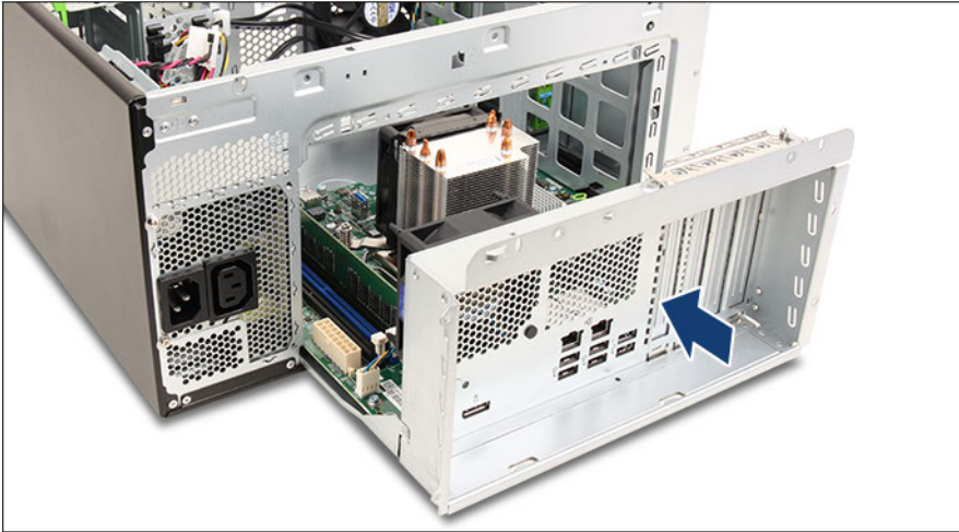
Figure 143: Installing the system board tray
