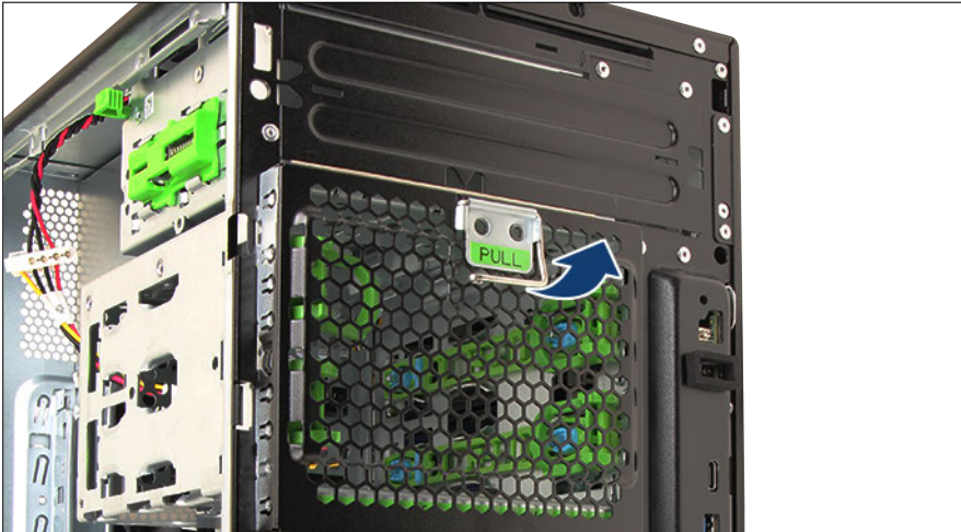
Figure 12: Pulling up the lever
