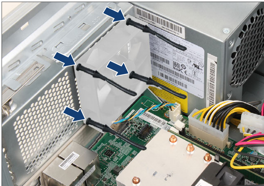
Figure 55: Inserting new rubber rivets
