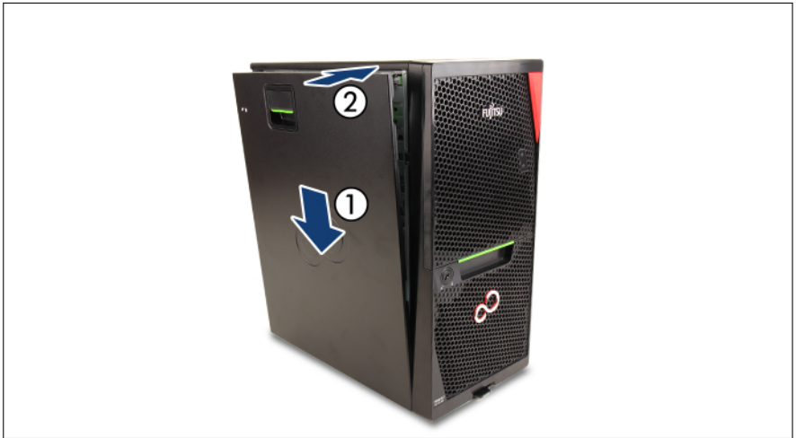
Figure 25: Installing the side cover
