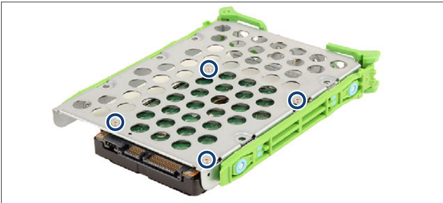
Figure 44: Detaching the 2.5-inch HDD from the 3.5-inch HDD carrier
