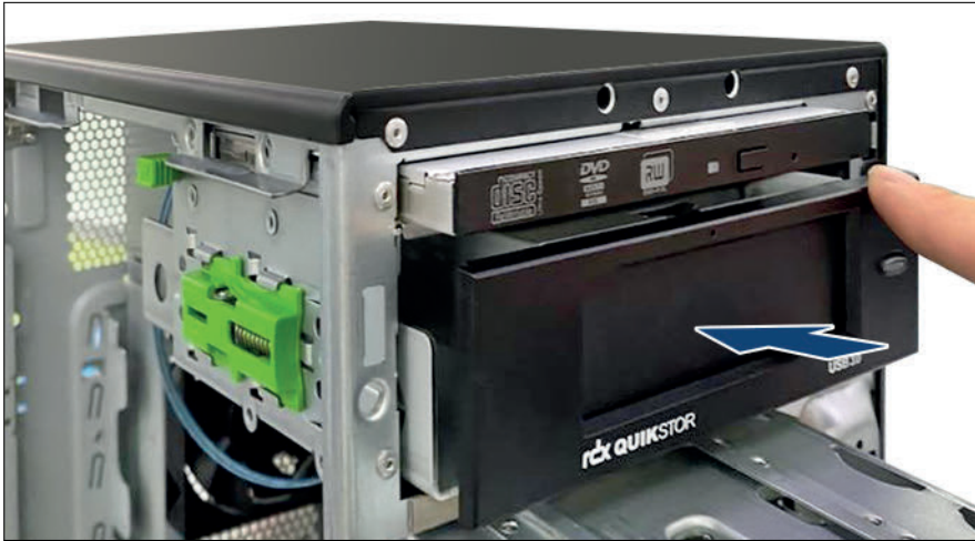
Figure 111: Inserting RDX backup drive into bay 2
