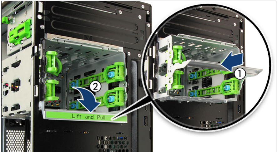
Figure 19: Pushing the HDD cage in and folding down the lever
