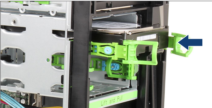
Figure 48: Inserting the 3.5-inch HDD
