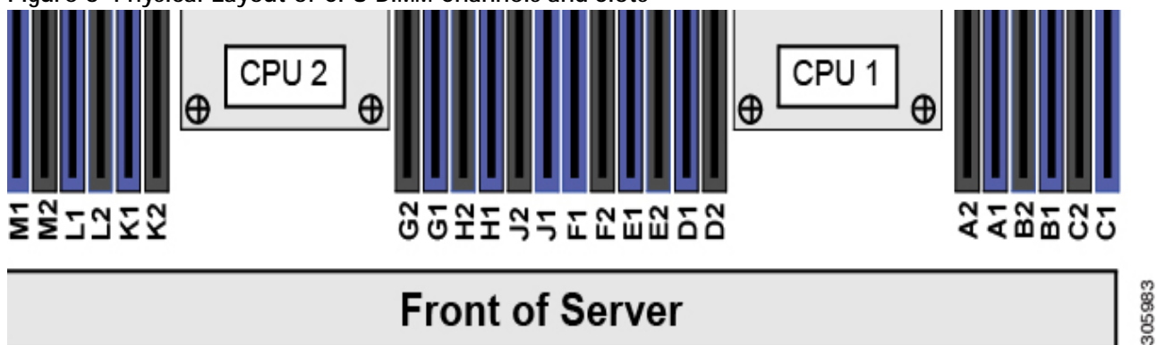
Figure 6 Physical Layout of CPU DIMM Channels and Slots
