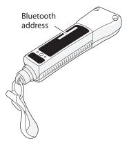
**SF51 Bluetooth Address:** The SF51 Bluetooth address is located in the upper right corner of the label on the back of the SF51.
