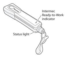
**SF51 Lights:** The status light turns green or red to indicate the status of the battery and scanning. The blue Intermec Ready-to-Work™ indicator turns on to let you know that the SF51 is ready to send data to your host Bluetooth device.
