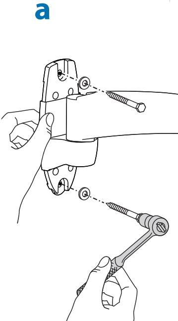
**CAUTION:** Make sure the wall mount bracket is level, flush and snug to the wall surface.
