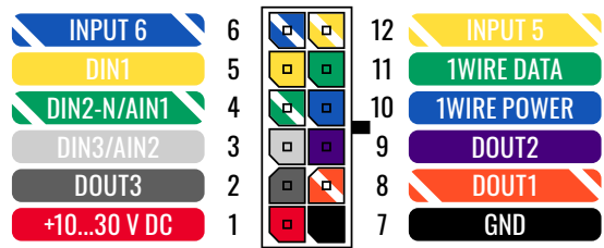
FMM230 2x6 socket pinout
