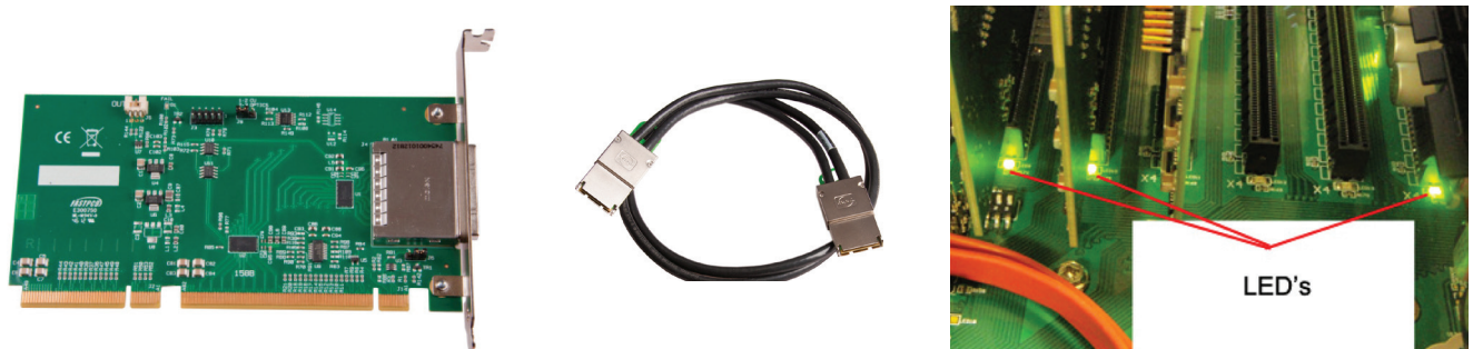
Figure 4-3. Pre-installed cards and appropriate cable to link them together.
