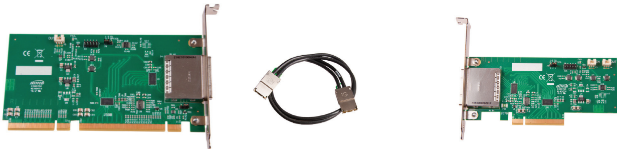
Figure 4-7. Pre-installed cards and appropriate cable to link them together.
