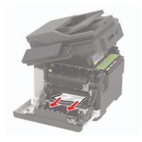
**3** Open the fuser access door, and then remove the jammed paper.
