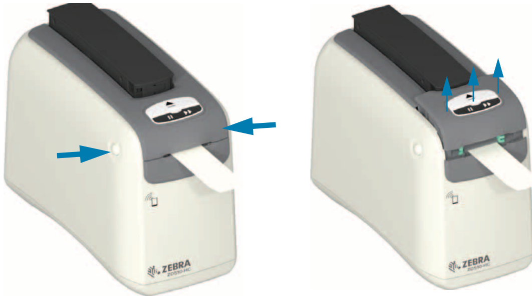
Figure 8 • Releasing Media Under the Upper Cover
