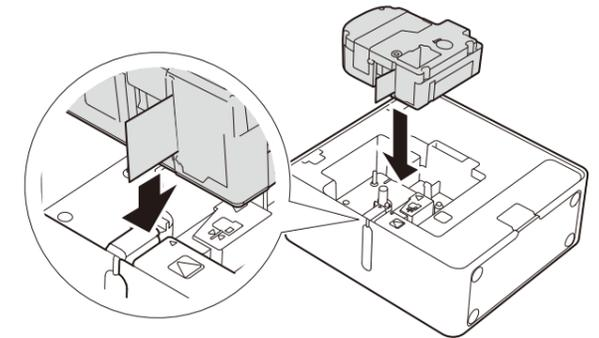
Place a tape cartridge. Press it firmly until it snaps into place.
