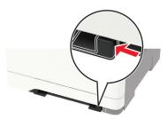
**2** Load a sheet of paper with the printable side facedown.
