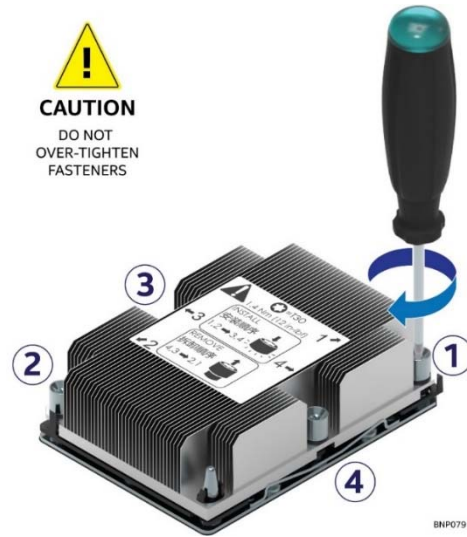
Figure 41. Installing the PHM
