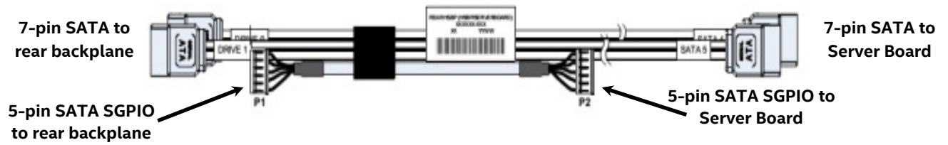
Figure 98. Rear HSBP SATA & SGPIO Cable Bundle
