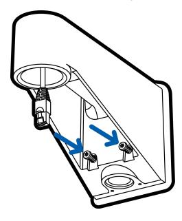
7. Loosely thread the lock nut onto the NPT adapter, then secure the NPT adapter into the pendant wall mount.
