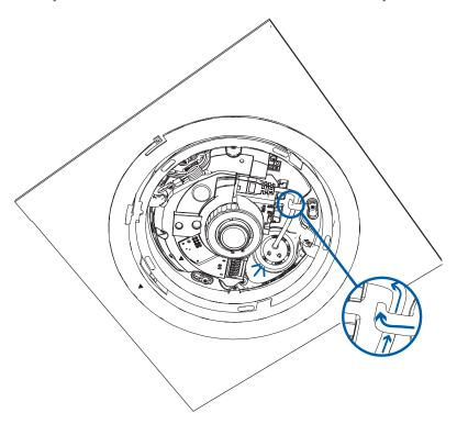
8. Use the cable clip to hold the Ethernet cable in the correct position.
