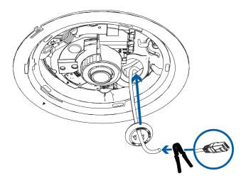
7. Install the grommet into the cable entry hole on the camera base. Make sure the grommet flange is securely seated on the inside and outside of the cable entry hole.
