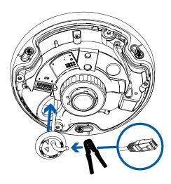
7. Push the rubber sealing grommet with the required cables into the cable entry hole on the camera base. The thread around the grommet should line up with the cable entry hole.
