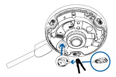
10. Push the rubber sealing grommet with the required cables into the cable entry hole on the camera base. The thread around the grommet should line up with the cable entry hole.
