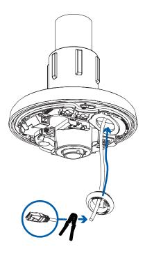
6. Push the rubber sealing grommet with the required cables into the cable entry hole on the camera base. The thread around the grommet should line up with the cable entry hole.
