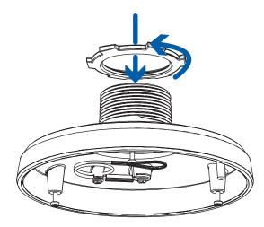
4. Apply thread seal tape to the NPT adapter and screw it into the pipe adapter.
