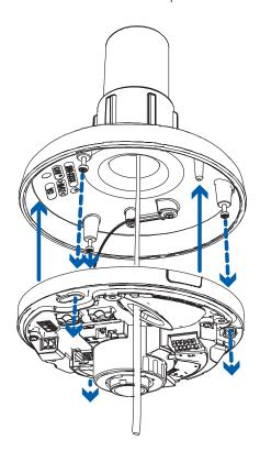
3. Twist the camera base clockwise until the posts come to the right end of the mounting slots.
