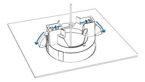
5. With your thumb on the outside edge of the mounting adapter and your forefinger on one of the orange clamp handles, pinch the clamp down until the clamp is secured.
