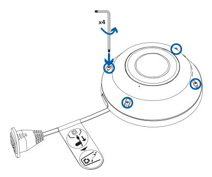
**Note:** Be careful not to scratch or touch the dome bubble. The resulting marks or fingerprints may affect the overall image quality. Keep the protective covers on the outside of the dome bubble until the installation is complete.
