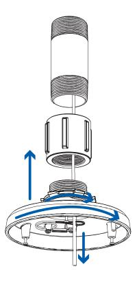
5. Carefully tighten the lock nut until the NPT adapter is secured to the conduit pipe.
