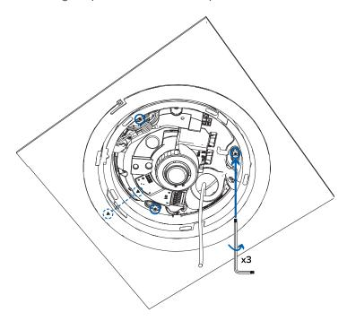
6. Pull the required cables through the rubber sealing grommet. For more information, see *Preparing the Cables* on page 13.
