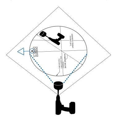
2. Insert the in-ceiling mounting adapter into the entry hole then pull the required cables through the adapter. Ensure the orientation arrow on the adapter is facing the same direction as it did on the mounting template.
