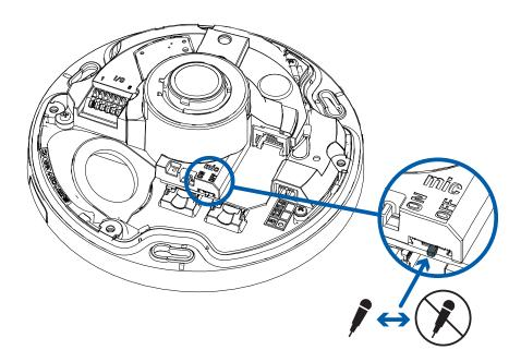
2. Slide the switch from the default OFF position to ON to enable the microphone.
