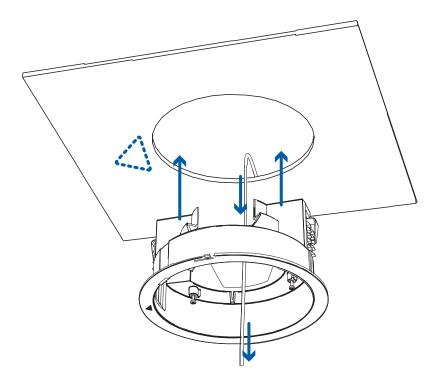
3. Pull off the elastic clamp retainer holding the clamps in place.
