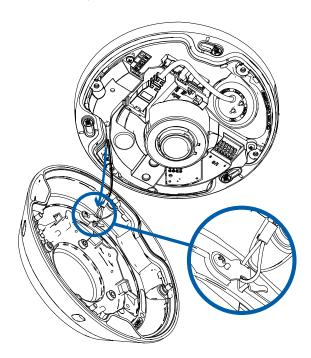
2. Attach the cover to the base and tighten the screws with the star-shaped screwdriver.
