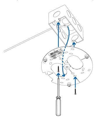
4. Pull the required cables through the electrcal box and a cable entry hole on the wall plate. Then feed the cables through the cable entry hole on the camera base.
