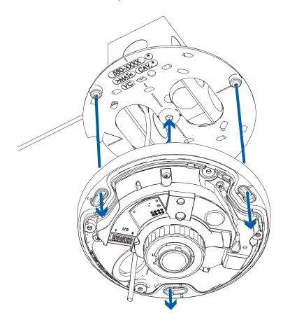
6. Twist the camera base clockwise until the posts come to the right end of the mounting slots.
