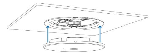
3. Rotate the cover clockwise while pushing up so that it clicks into place.
