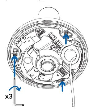
5. Pull the required cables through the rubber sealing grommet. For more information, see *Preparing the Cables* on page 13.
