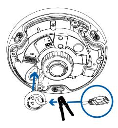
9. Push the rubber sealing grommet with the required cables into the cable entry hole on the camera base. The thread around the grommet should line up with the cable entry hole.
