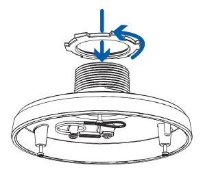
8. Carefully tighten the lock nut until the NPT adapter is secured to the wall mount.
