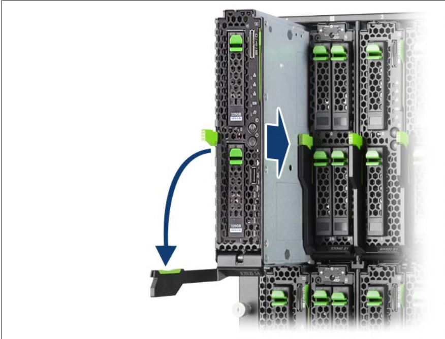
Figure 3: Installing the server blade
