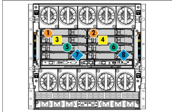
To support network connections for specific signals, install an interconnect module in the bay corresponding to the FlexibleLOM or mezzanine signals.
