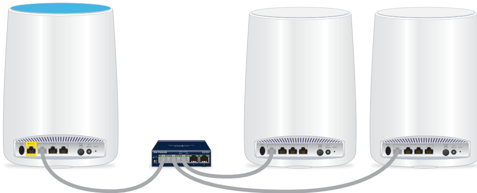
Figure 3. Ethernet backhaul connection using a switch
