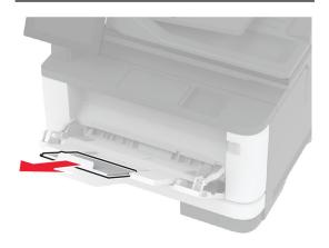
2 Flex, fan, and align the paper edges before loading.
