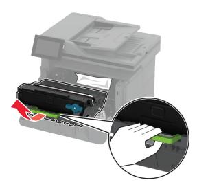
Warning—Potential Damage: Do not expose the imaging unit to direct light for more than 10 minutes. Extended exposure to light may cause print quality problems.
