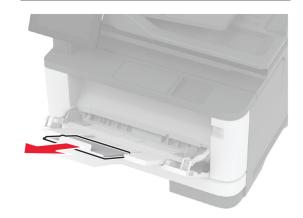
**10** Flex, fan, and align the paper edges before loading.
