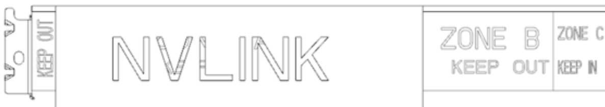
Figure 4. NVLink Connector Keep Out Area – Top View
