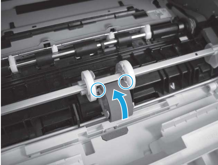
Figure 9-13 Install the roller
