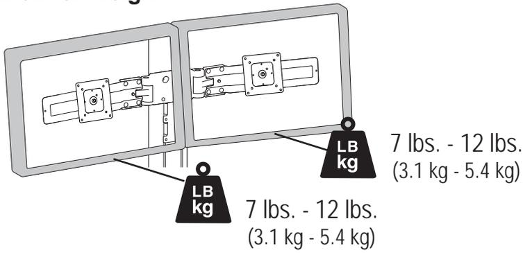
Total weight of monitors when mounted needs to be 14 lbs - 24 lbs (6.2 kg - 10.8 kg)
